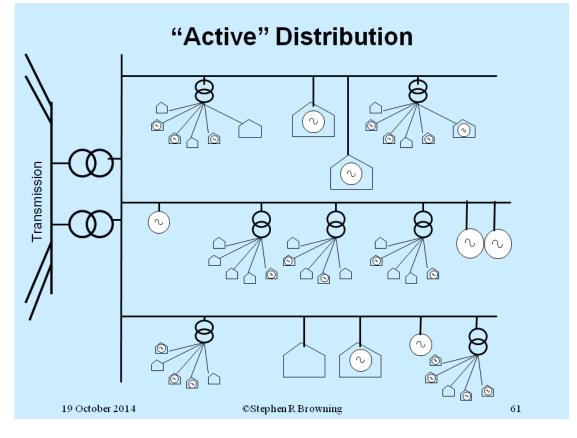
At domestic level we have Micro CHP, PV or Wind technology. PV is expensive, due to local turbulence Wind gives low yield at roof height and CHP systems (boiler + heat recovery turbines) are still being commercialised. However, the penetration of Micro Generation is forecast to increase.
