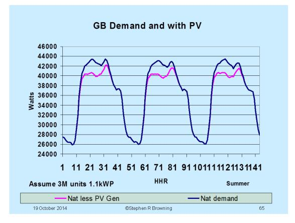
On commercial premises, maximum PV output occurs during the building maximum demand period and is synergistic with any electrical cooling load.
