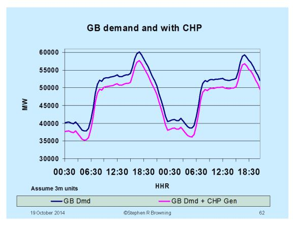
With a cold, uniform external temperature the CHP will run continuously day and night. This is not the most efficient way to reduce fossil generation output.
